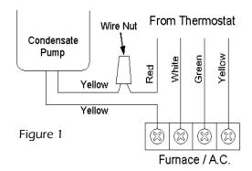
LOW VOLTAGE—AUXILIARY SAFETY SWITCH— Units designated with an 'x' in the model number (L4x) have a built in safety switch. Connect the leads of auxiliary safety switch to the thermostat control circuit of the air conditioner/furnace. This will disrupt the thermostat demand in a high water condition. (Figure 1)
