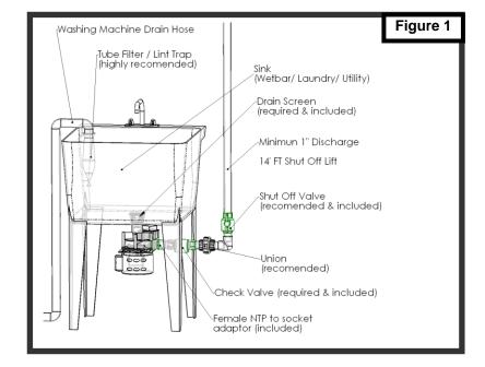
! NOTE Sinks will only allow 5-6 gallons-per-minute (GPM) of water to pass through the drain into the pump. When the pump is lifting water to a height of 8 feet, the LTA pump will remove 23 GPM. This causes the pump to turn on and off frequently, or "cycle". The shut off or balancing valve acts to adjust or "balance" the discharge flow to match the inlet flow being let into the pump from the sink and reduces pump cycling. Adjust pumps as follows to minimize cycling:
