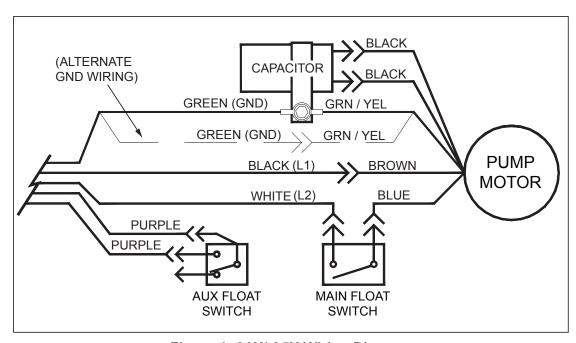
Figure 1. A3X/ A5X Wiring Diagram
